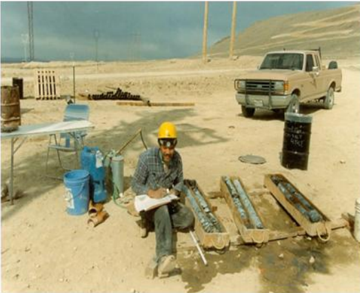
Logging original metallurgical 4 inch core for the Lone Tre Mine, circa 1990.
