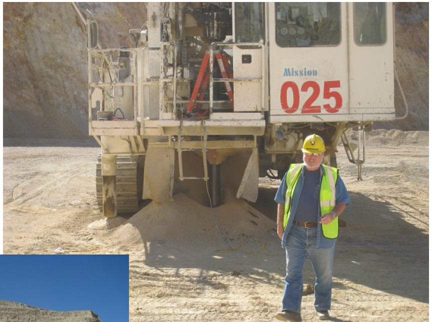
Shaddrick, can't you read the itty bitty keep out sign? But where's the rocket? Atlas Copco Pit Viper 235 sans through-the-deck rocket sampler.
